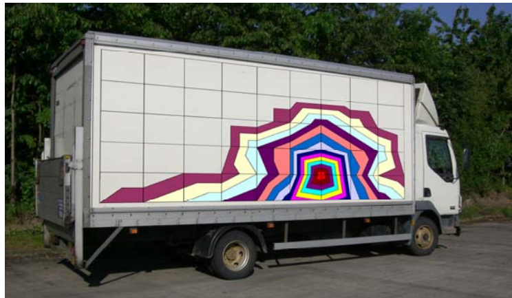
Figure 8: Dose rate map overlay projected onto target vehicle
